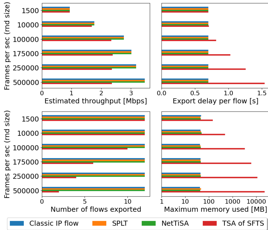
Figure 4.9: Results of performance and memory requirements comparison using Spirent test server. The SFTS acronym in the legend stands for Single flow time series .
